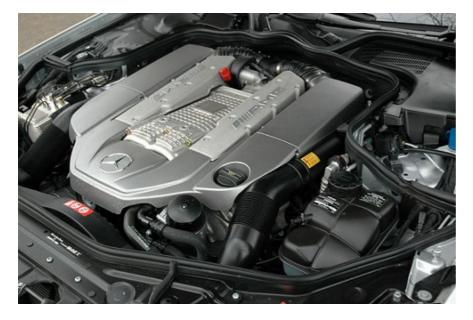
The power maxes at 6,100 rpm but it's the 700 Nm of torque from 2,650 - 4,500 rpm that produces the performance truly making the supercharged V8 engine one of the best out there. It's never very noisy, but burying the foot to the floor will elicit a droning roar akin to a WW2 fighter on overboost.
